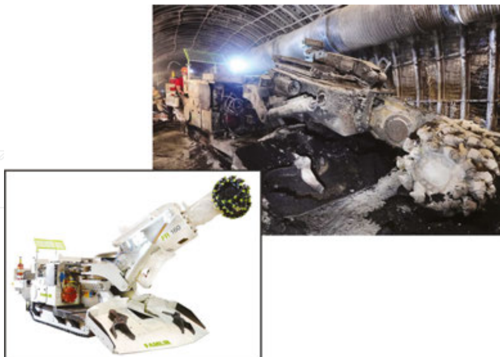
Figure 1. Boom-type FR 160 roadheader designed for drilling dog headings in underground mines and tunnels in civil engineering [6].
