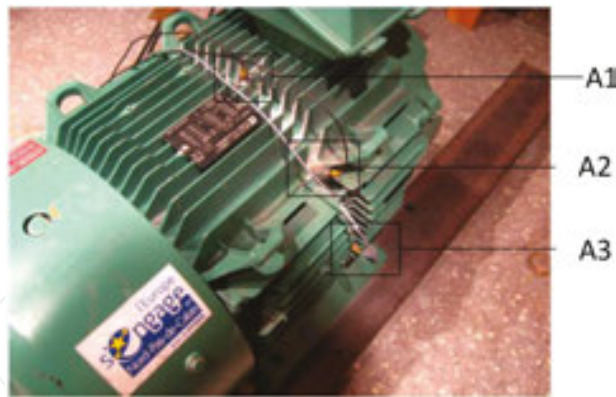
Figure 20. Positions of the accelerometers on M1.
