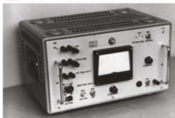
Figure 39. Apparatus for a speed control of tape passage.
