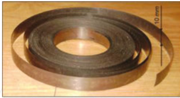
Figure 49. Segment of multilayer Nb/D16 tape.
