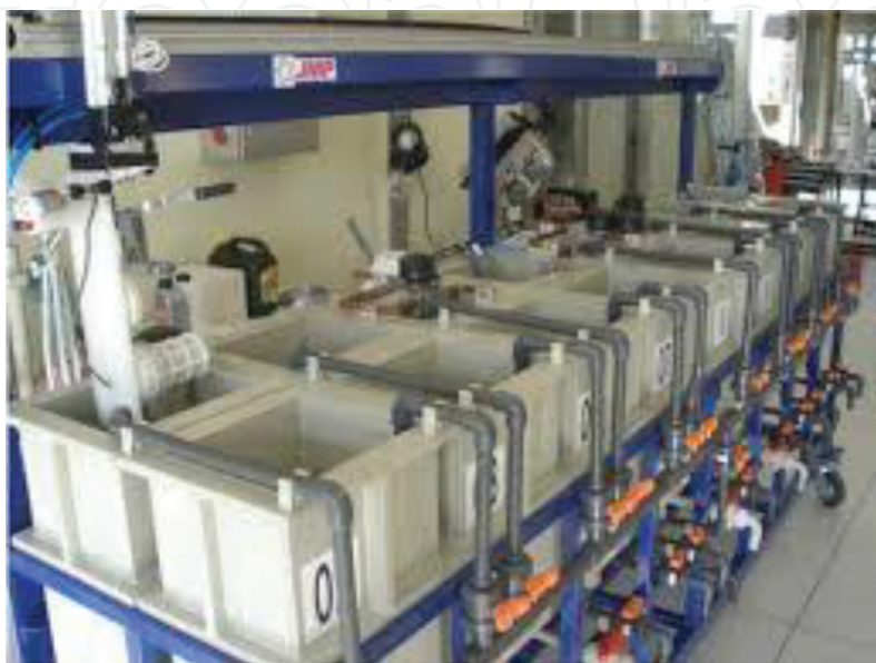
Figure 4. A chrome plating pilot plant part of the IONMET consortium activities [80].
