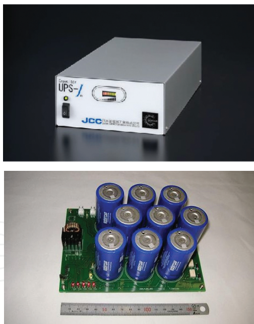
Figure 1. EDLC-based uninterruptible power supplies (UPSs).
