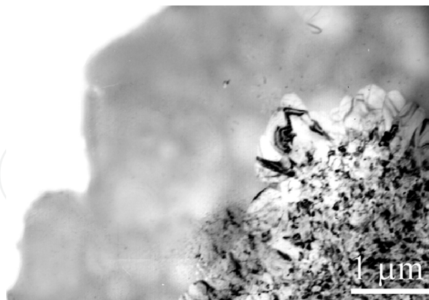
Figure 19. Microstructure of annealed and partially crystallized in-situ \text{Fe}_{83}\text{B}_{10}\text{P}_7 alloy.
