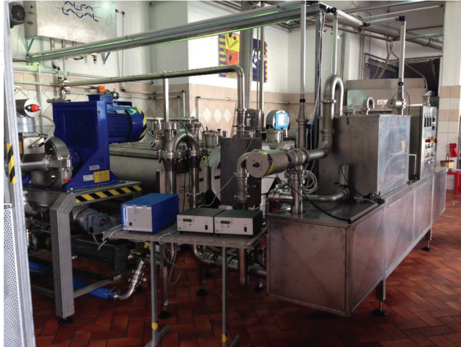
Figure 2. The sono-exchanger system and the three drivers, which provide the periodic signals (Colletorto, Italy, Aloia farm).
