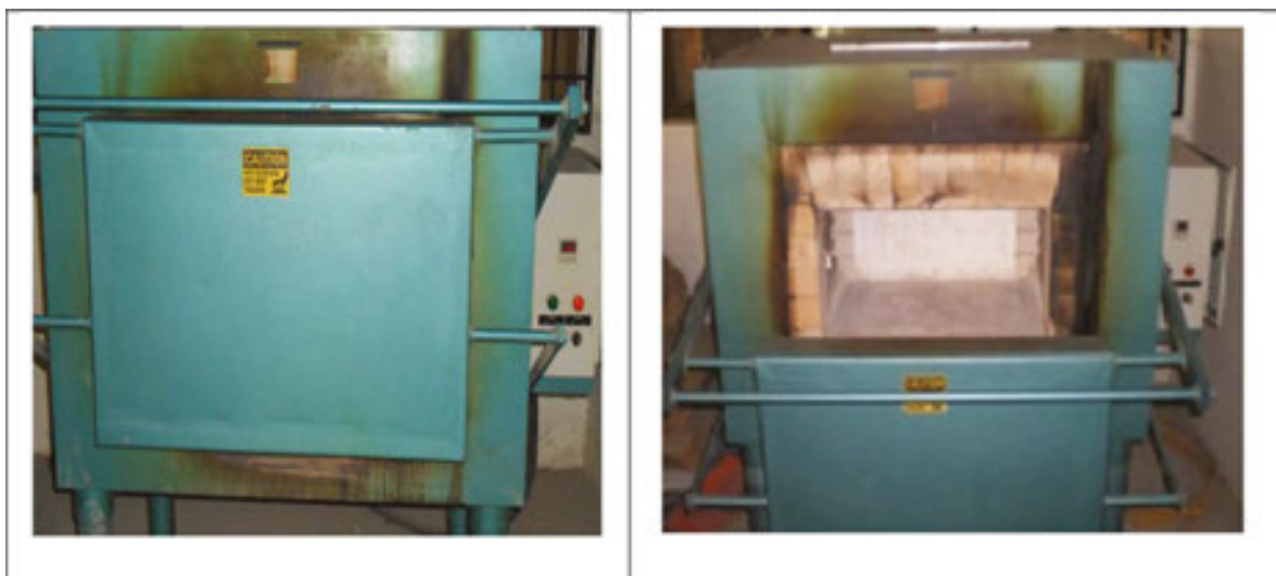
Figure 1. Automatic electric furnace used to heat concrete specimens.
