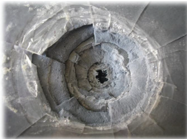
Figure 13. Crater originated in the double ceramic plate.
