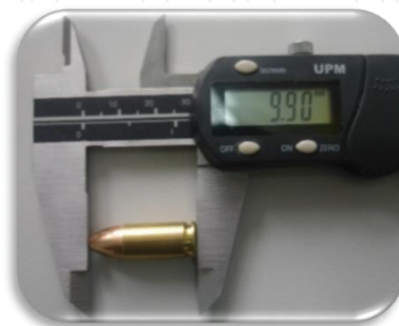
Figure 5. Longitudinal dimensioning of the projectile used.
