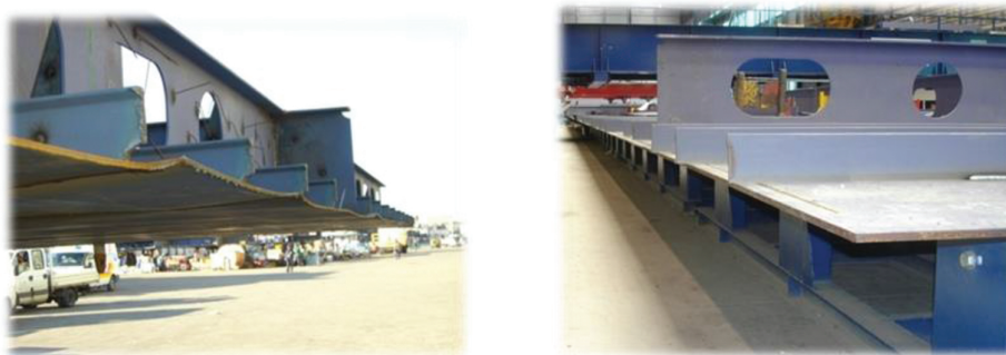
Figure 23. Comparison of MAG welded ship body section (left) with HLAW case (right).
