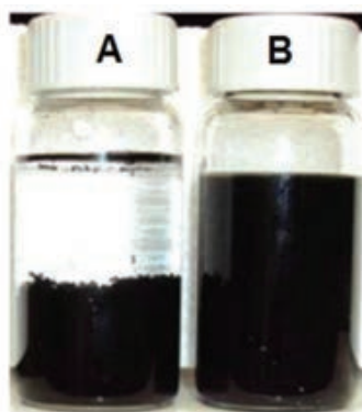
Figure 1. Nanofluid prepared by dispersing MWCNTs in deionized water (A) shows that MWNTs deposited at the bottom of the container and (B) shows that MWNTs maintain good dispersion: From Ref. [43].
