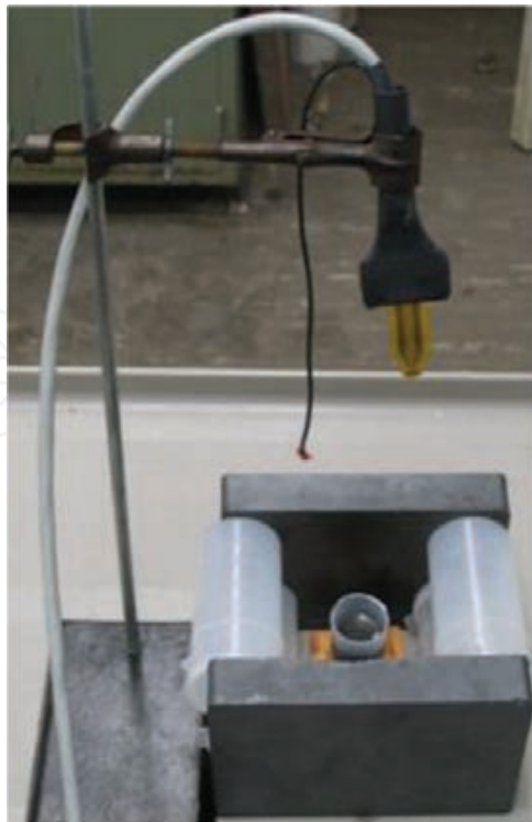
Figure 7. Experimental setup for measuring TC under application of a magnetic field. From Ref. [70].
