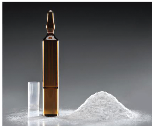
Figure 3. The PMMA bone cement is activated by mixing powder and liquid components.
