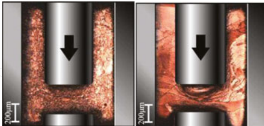
Figure 30. Microstructures of the microformed parts in microdouble-cup extrusion with different grain sizes. (a) 20 and (b) 150 \mu\text{m} [33].
