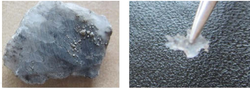
Figure 9. Thin film of hydroxyapatite on the salt after heated/thin and flexible film of HA.
