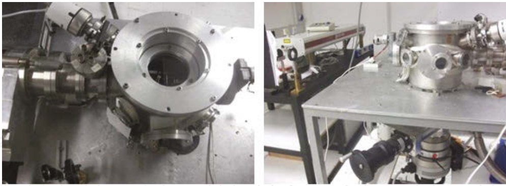
Figure 13. PLD experimental setup.
