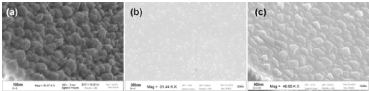
Figure 10. Zn film on Ru deposited (a) at room temperature and rate of 0.02 nm/s, (b) room temperature and 0.1 nm/s, and (c) at 100°C at 0.05 nm/s.
