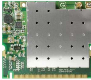
Figure 4.1: Wi-Fi Module containing 802.11p/DSRC Standard [83]
