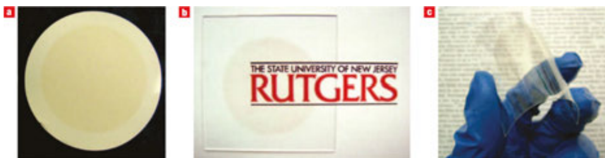
Figure 1. GO film obtained via the vacuum filtration method. (a) GO film on filter paper. (b) GO film on glass. (c) GO film on polyethylene terephthalate (PET). Reprinted by permission from Macmillan Publishers Ltd: Nature Nanotechnology (3:270), copyright (2008).[8].
