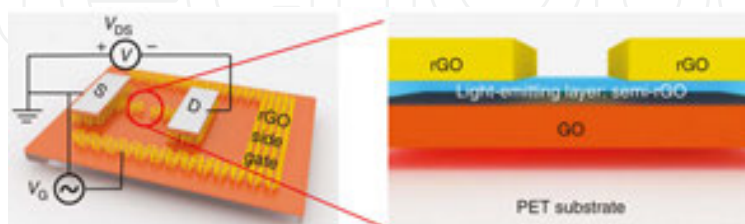
Figure 22. Device structure of the graphene light-emitting device. The semi-rGO layer functions as the light-emitting layer. Reprinted from Ref. [15] (CC BY 4.0).
