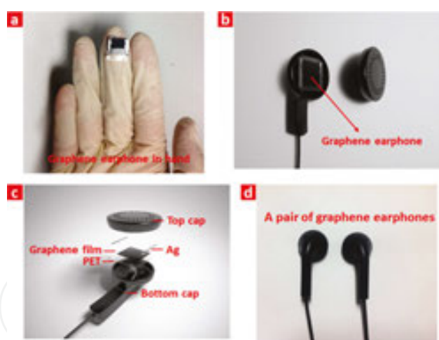
Figure 13. Packaged graphene earphone. (a) Graphene earphone in hand. (b) Graphene earphone after packaging. (c) The 3D assembled structure of the graphene earphone. (d) A pair of graphene earphones. Reprinted with permission from ACS Nano 8:5883. Copyright (2014) American Chemical Society [12].
