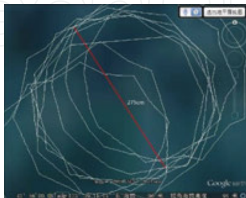
Figure 12. The minimum turning circle (radius 1.375 m).
