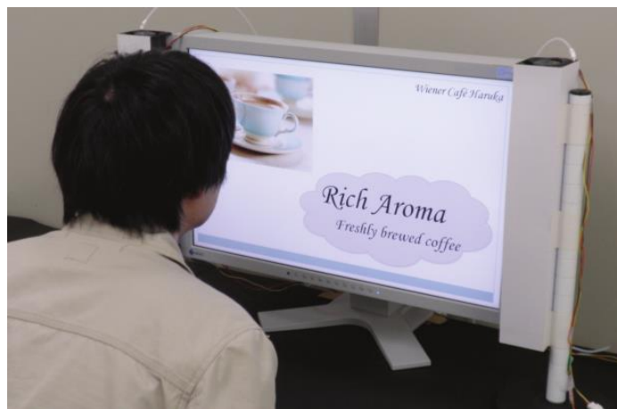
Image 5 User testing the Smelling Screen to sense the aroma of coffee (Matsukura et al., 2013)
