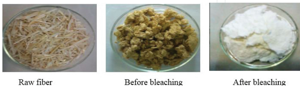
Figure 6. Image of raw wheat straw fiber, and its pulp before and after bleaching.
