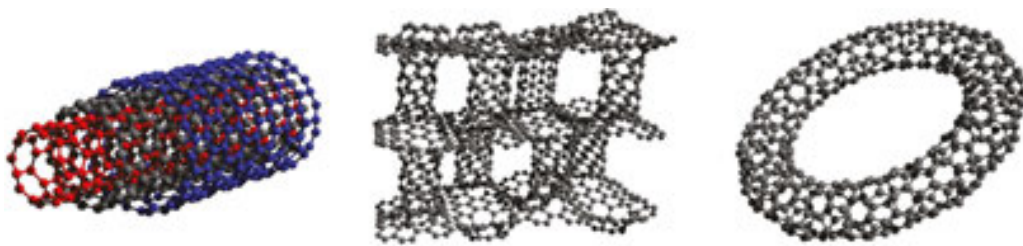
Figure 5. Less common forms of the graphene nanostructures: triple-walled nanotube (left), pillared graphene (middle), nanotoroid (right).
