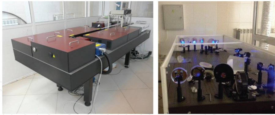
Figure 7. (a) Femtosecond Ti:sapphire front end. (b) Prism pair arrangement.
