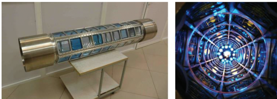
Figure 9. (a) Laser cell of the \text{XeF}(\text{C-A}) amplifier. (b) Inside view of the laser cell with the mirror unit.
