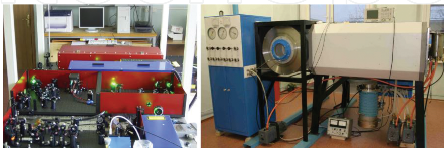
Figure 4. THL-30: Photographs of the Ti:sapphire front end (left) and XeF(C-A) amplifier (right).
