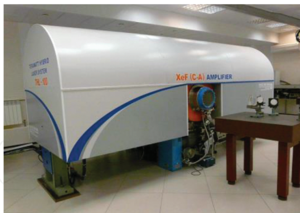
Figure 8. General view of the XeF(C-A) amplifier.
