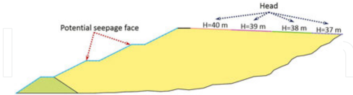
Figure 9. Boundary conditions and discretization model for the tailings dam with Seep/W [41].
