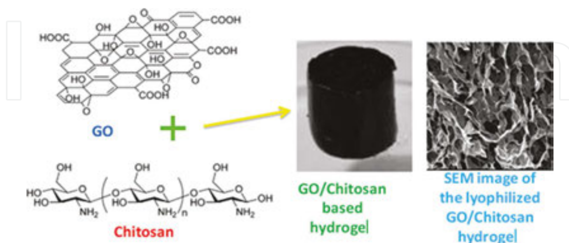
Figure 7. Photograph of GO/chitosan hydrogel and its SEM image. Reproduced from [107] with the permission from RSC.
