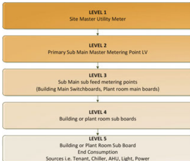
Figure 1. Large building and campus electricity smart meter architecture.
