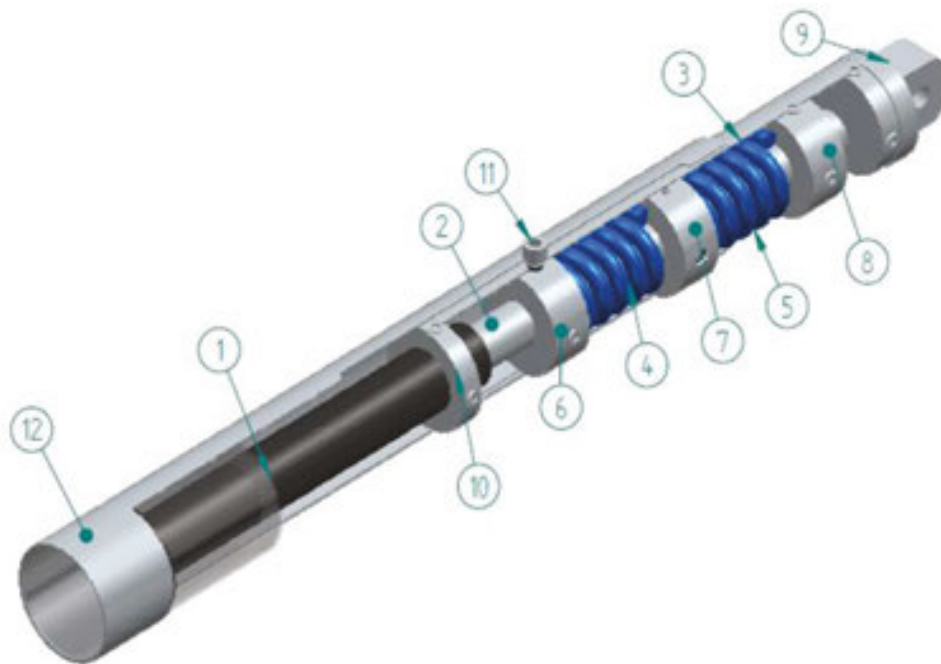
Figure 17. Actuator's components: (1) hydraulic cylinder; (2) movable rod; (3) base tube; (4) and (5) springs; (6), (7) and (8) low friction sliding cylinders; (9) load terminal; (10) connection guide; (11) guide bolt; (12) encapsulation tube.
