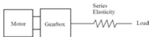
Figure 1. Series elastic actuator schematic (Williamson, 1995).
