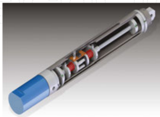
Figure 12. Actuator final design with internal components.
