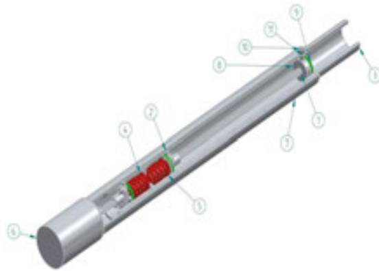
Figure 10. First prototype showing internal actuator components: ball screw (1); ball nuts (2); movable arm (3); springs (4, 5); motor & gearbox (6); base tube (7); bearing screw (8); O-ring (9); Allen screws (10); guide ring (11).
