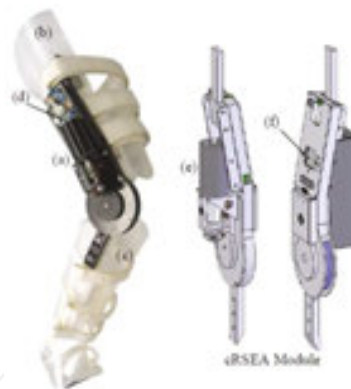
Figure 7. Proposed exoskeleton for knee assistance. (a) Rotary SEA module, (b) a thigh brace, (c) a calf brace, (d) a motor driver, (e) a DC motor, and (f) an controller (Kong et al., 2010).
