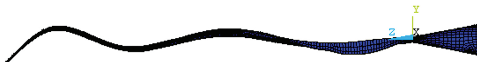
Figure 8. Bending mode following torsion mode of the 660 (kW) composite wind turbine blade.
