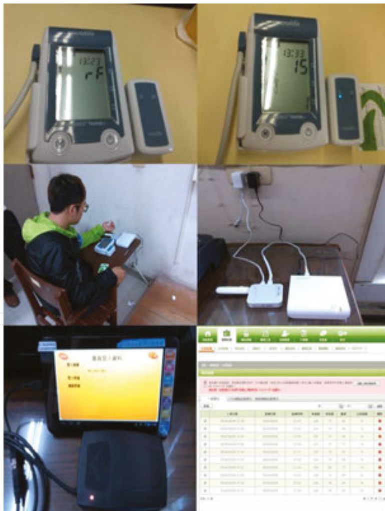
Figure 8. A learning tool developed by Microlife Corporation for 3G mobile agent and cloud-based multiuser real time BP measurement system.
