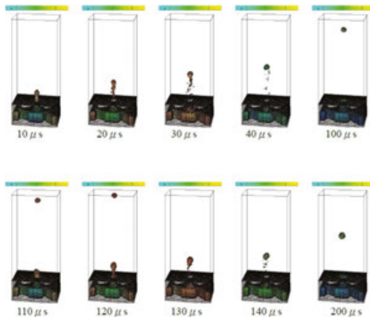
Figure 15. Numerical simulation of DNA in the nozzle diameter 30\ \mu\text{m} and 50\ \mu\text{m} thickness tapered dual channel injection chamber to 10\ \text{kHz} operating frequency, three-dimensional side view, in 10, 20, 30, 40, 100, 110, 120, 130, injection of the case 140 and 200\ \mu\text{s} .
