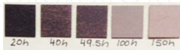
Figure 9. Expanded view of the 530°C gradual transition from black to grey oxide.
