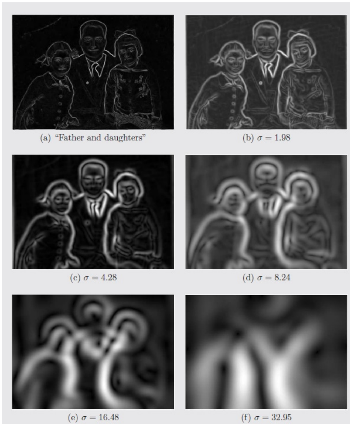
Figure 3.2: As the scale of the filter increases, transition between regions becomes less and less sharp
