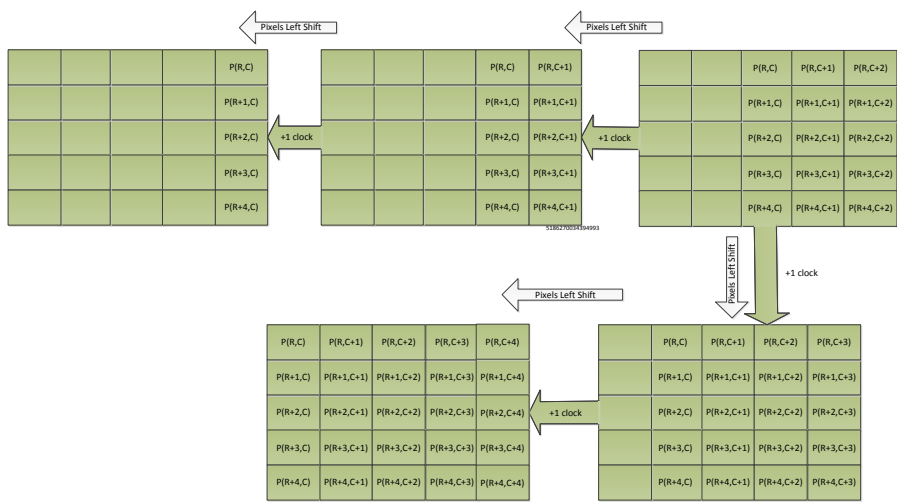
Figure 4.8: Mask shift process in the Gaussian Operator. P = pixel, R = row and C = column
