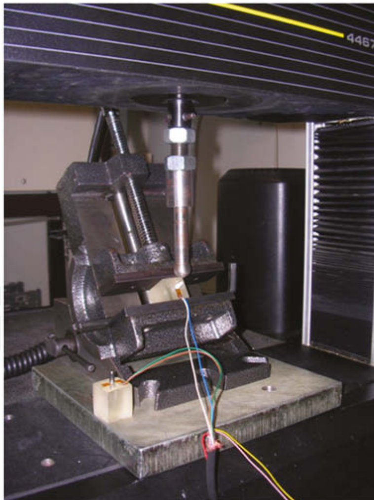
Figure 4. The experimental validation of numeric model of a zirconia implant (from Mobilio 2013).
