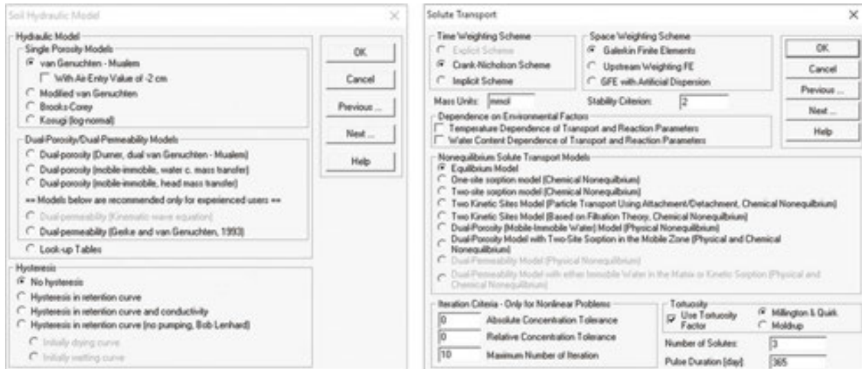
Figure 9. Snapshot of soil hydraulic (left) and solute transport (right) selection window in HYDRUS-1D.
