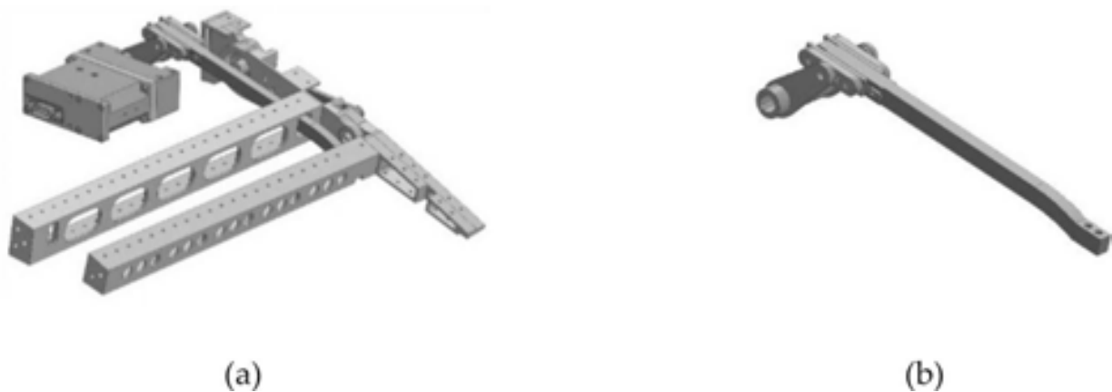
Figure 15. Actuation system final architecture with high rigidity linear guide.
