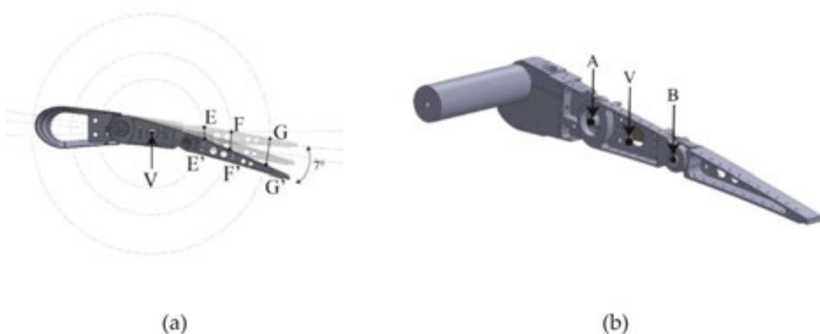
Figure 13. Circular trajectories of sample points (E, F, and G) during morphing (left) and position of hinges A, V, and B (right).
