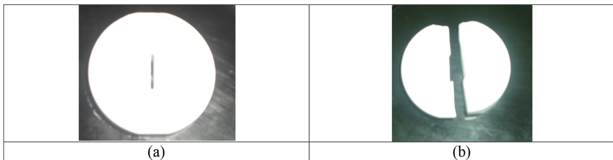
Figure 15. (a) CSTFBD before testing and (b) failure mode of CSTFBD specimens.
