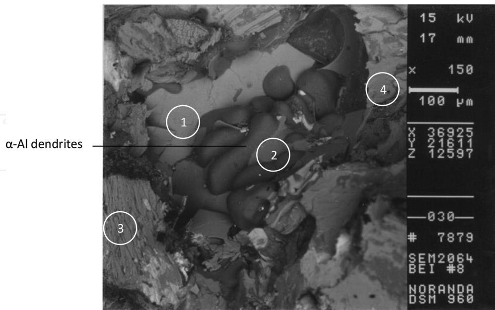
Figure 17. SEM micrograph showing the effect of porosity participating in the fracture behavior of alloy 319.2 (0.8% Fe, DAS 83 \mu\text{m} , modified).
