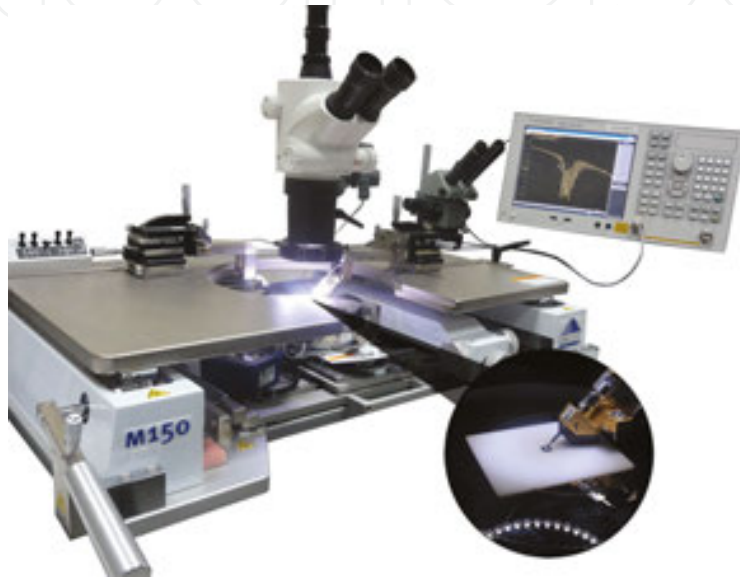
Figure 6. Experimental setup: E5071C network analyzer, M-150 probe station, and studied diamond-based PLS.
