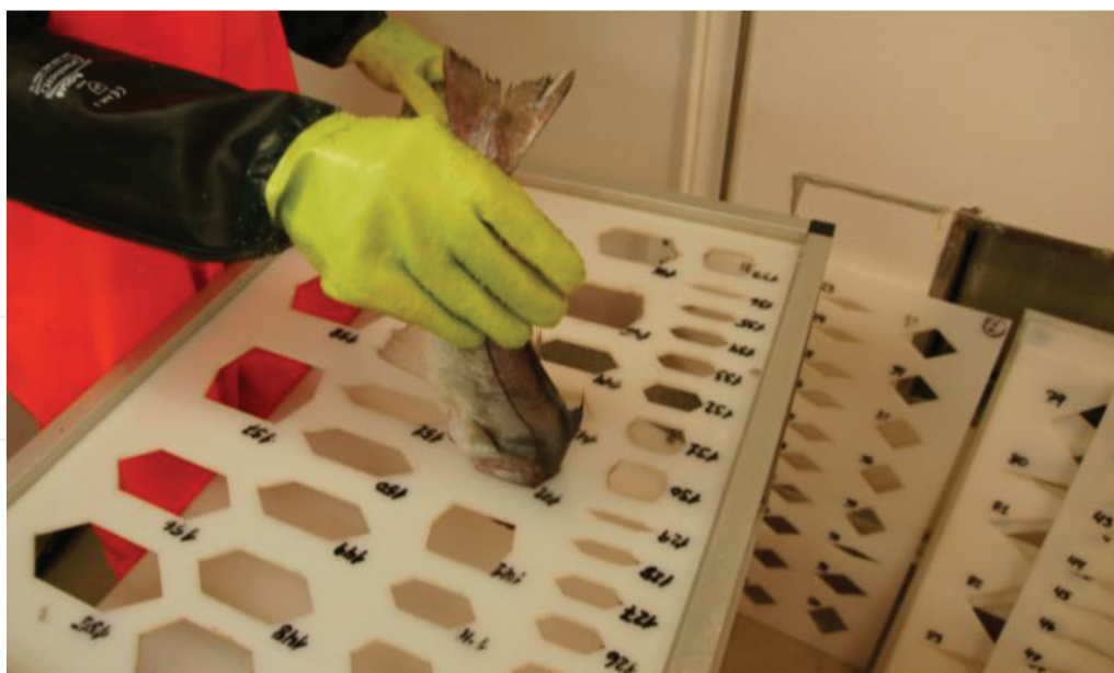
Figure 8. Illustration of the fall-through procedure on haddock ( Melanogrammus aeglefinus ). Each interchangeable plate contains a number of different mesh shapes where each fish is tested. All fish included in the study need to be tested in all meshes.
