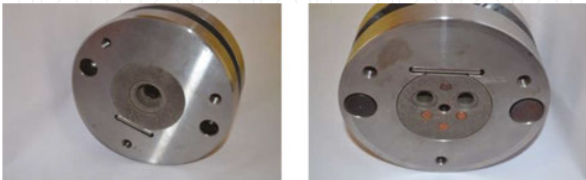
Figure 11. Active elements of moulds made by SLM mounted onto the plates manufactured at Plastor S.A. company from Oradea.
