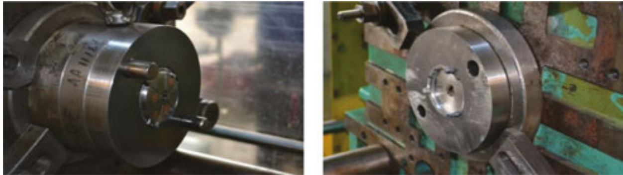
Figure 16. Injection moulding tools mounted on the Arburg 370 CMD 800-325 testing machine from Plastor SA Oradea.
