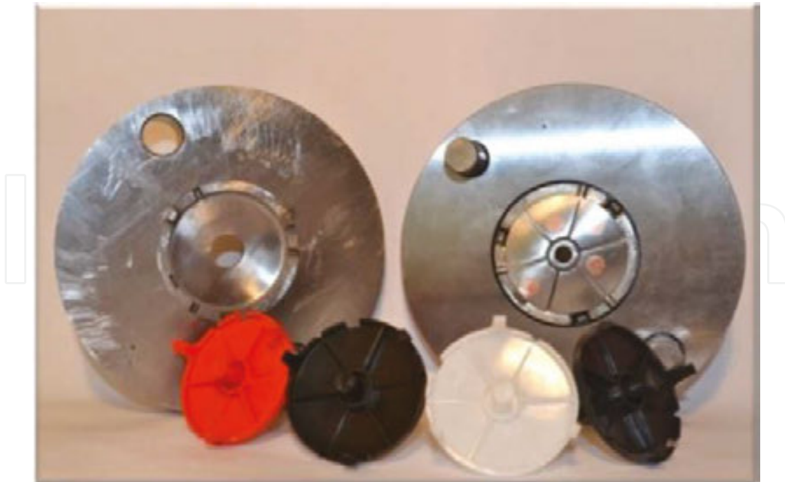
Figure 17. Injected plastic materials obtained at Plastor SA Oradea using the injection moulding tools made by SLM.
