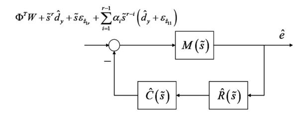
Figure 1. Repetitive controller and stabilizing compensator.
