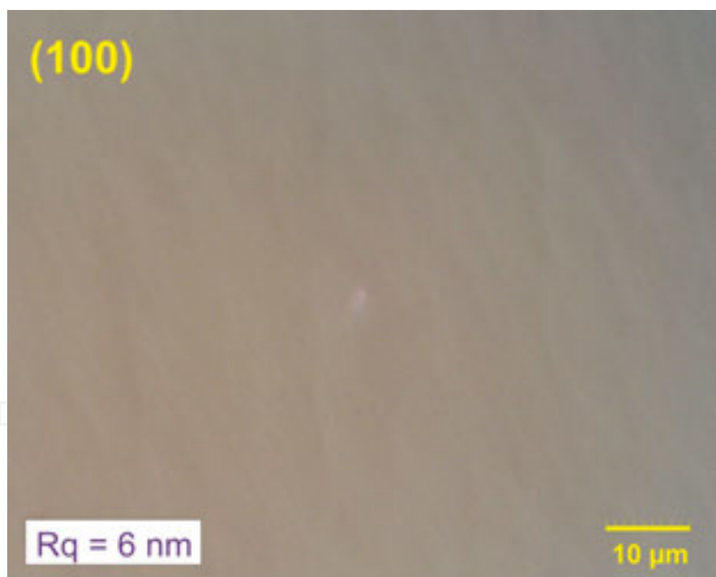
Figure 7. The example of surface morphology of obtained (100) oriented HgCdTe layer.
