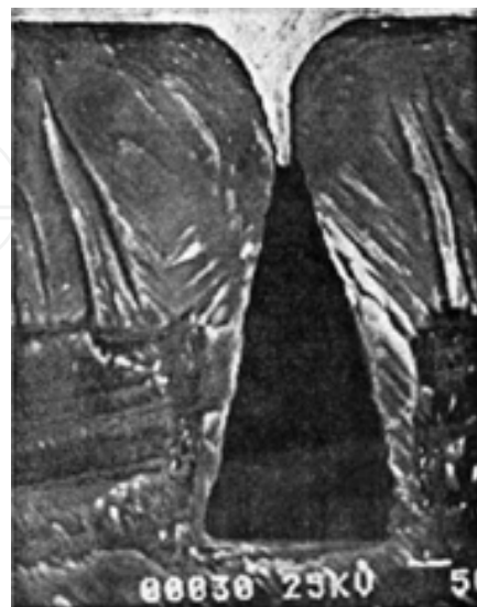
Figure 5. A vapor-deposited micro-grooved heat pipe [17].
