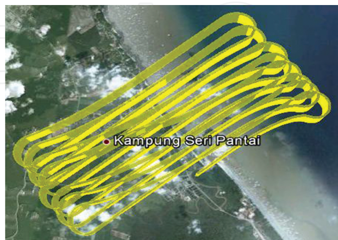
Figure 10. Navigation path of the real-time GPS-aided SINU system experiment on a UAV in Google Earth.
