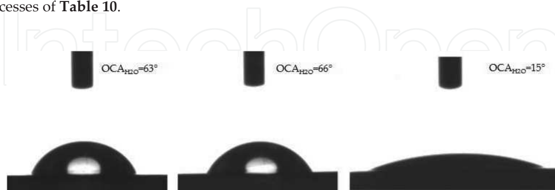
Figure 10. OCA_{H_2O} images for the first three processes listed in Table 12 , on Si.
