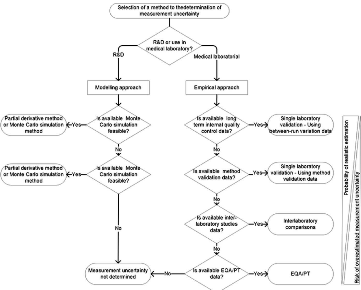
Figure 6. Flow chart to select a model for the determination of measurement uncertainty in a medical laboratory.
