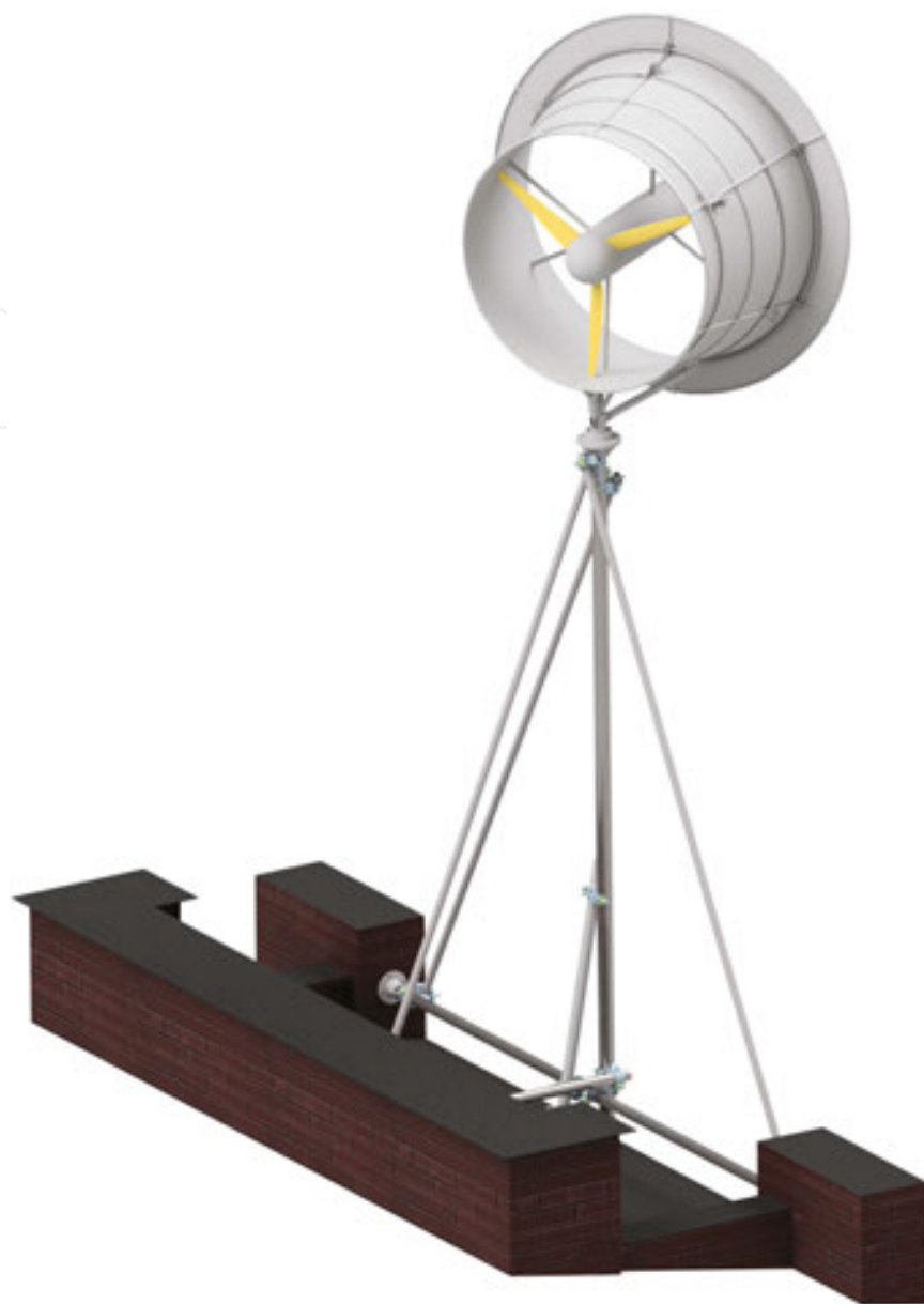
Figure 6. Roof-mounted SWT equipped with the diffuser.
