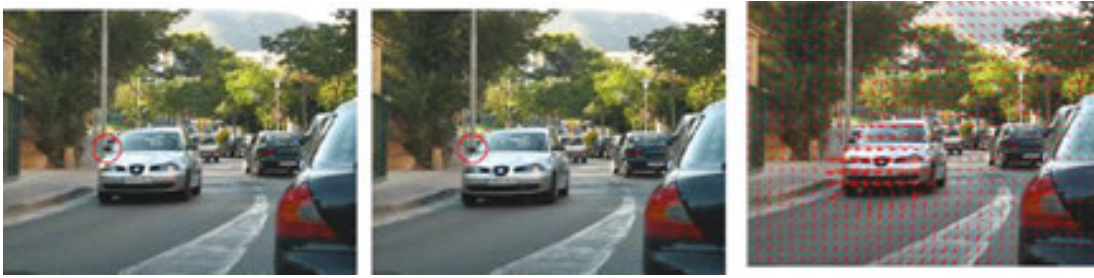
Figure 2. Optical Flow Representation in a Sequence of Images [19]. (a) Frame 43 of the Camera Motion Sequence . (b) Frame 44 of the Camera Motion Sequence . (c) Optical Flow Result.
