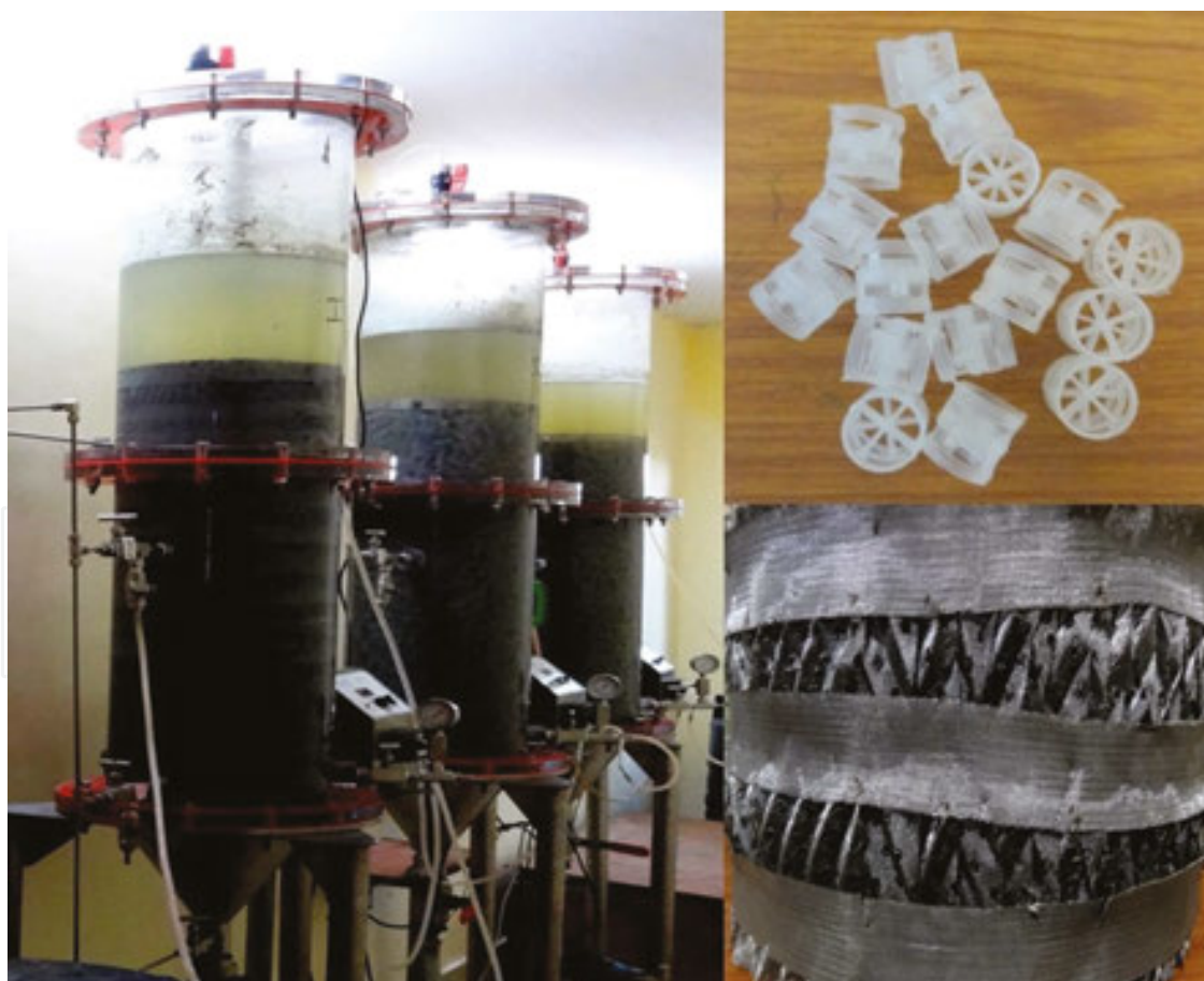
Figure 1. 220-litre packed bed bioreactor for soluble sulphate removal with steel and polypropylene immobilization substrate with defined surface area for bacterial biofilm formation.
