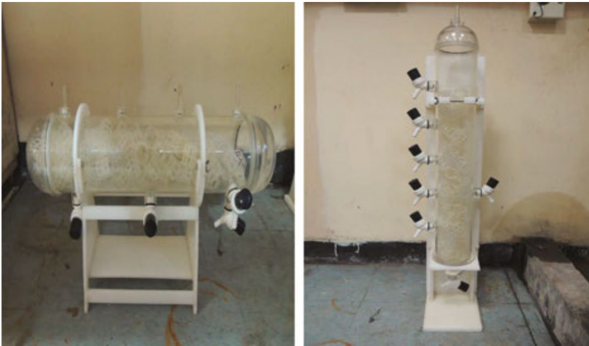
Figure 10. (a) Modified design of packed bed bioreactor. (b) Actual bioreactors constructed using plastic material.
