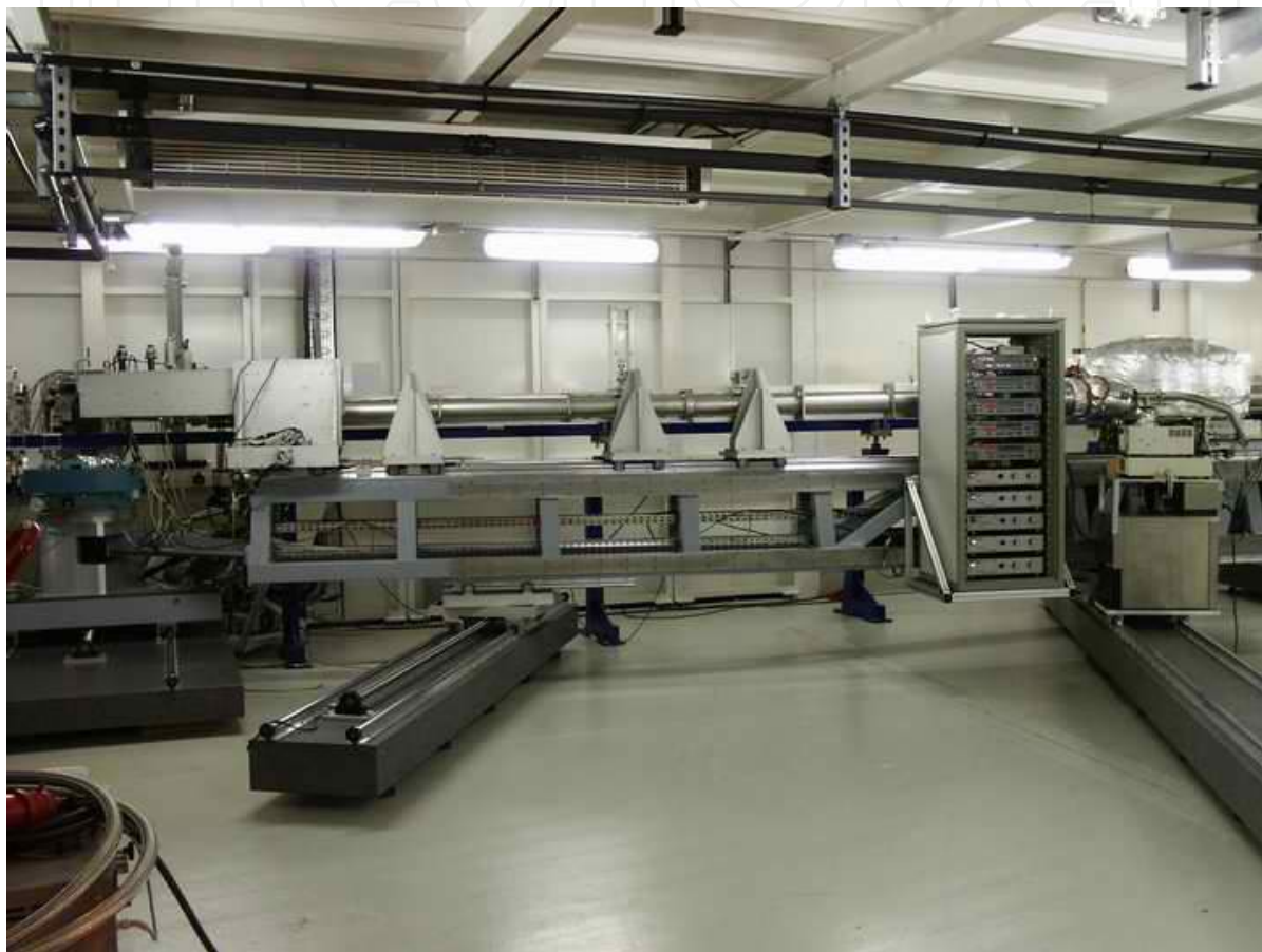
Figure 7. The ID28 beamline's spectrometer arm of at ESRF (from the ID28 beamline's website, courtesy of A. Bosak)
