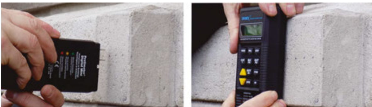
Figure 6. Left: Pin moisture meter (Protimeter), right: pinless moisture meter (Tramex).
