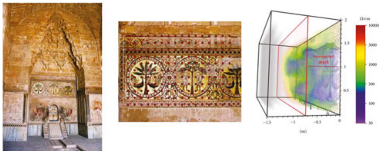
Figure 17. Frontal wall of the Fountain Room of the Arabian Zisa Palace in Palermo (left); position of the 176 potential electrodes (centre) and 3D inversion model of the acquired data (right). Adapted from Cosentino et al. [4].
