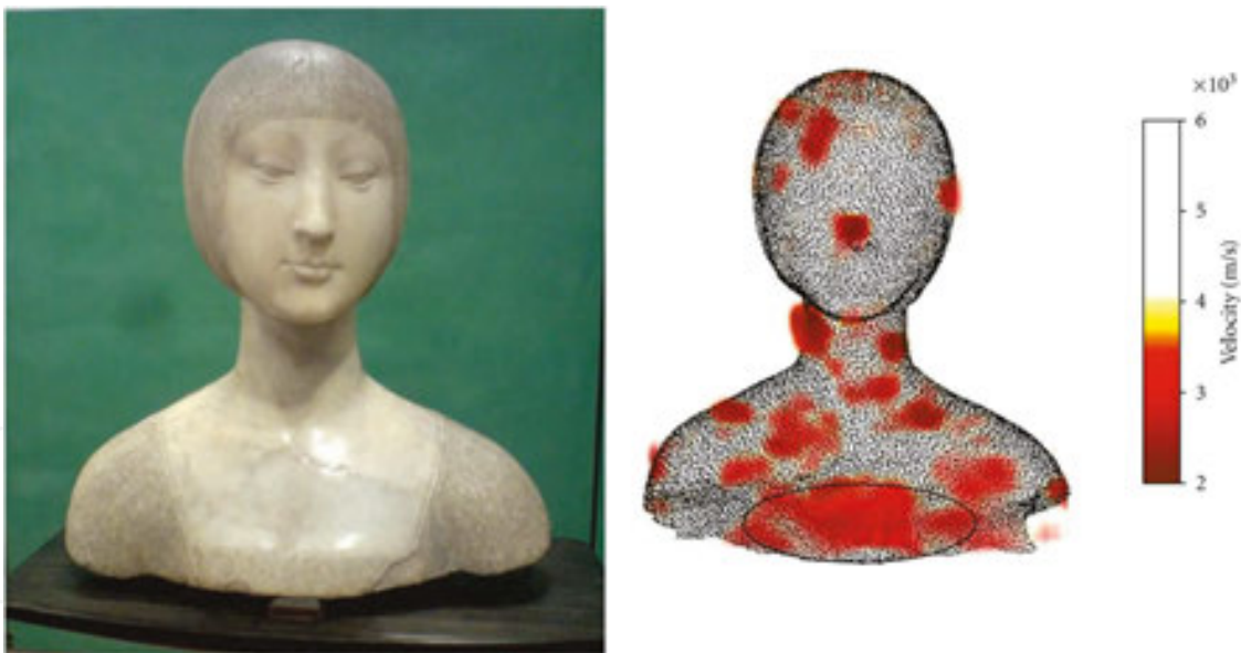
Figure 13. 3D ultrasonic travel time tomography on the Eleonora d'Aragona statue. Adapted from Cosentino et al. [4].
